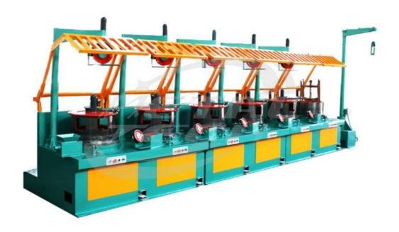
Wheel type wire drawing machine is one of many types of wire drawing machine, but its application range is the most extensive. By adopting international and domestic advanced technology, Metal Tech's wheel type wire drawing machine can meet the specific needs of different customers, and can draw the wire to the specified wire diameter according to the customer's requirements. In addition, the Metal Tech wheel type wire drawing machine is cost-effective, fast, and has low
